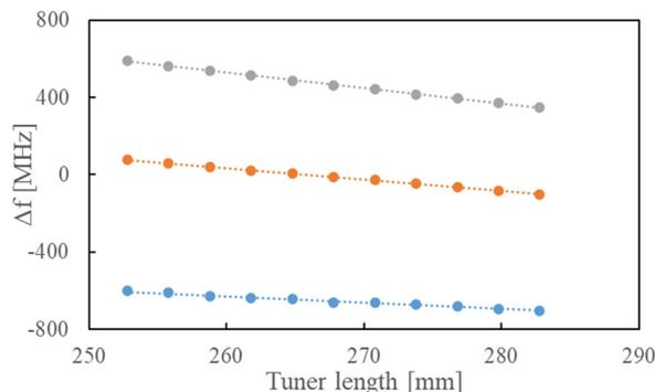
Figure 2: Three resonances (showed as three lines in the plot) in the tuner that are adjacent to 1.4 GHz, with x axis the tuner length and y axis the frequency away from 1.4 GHz.
