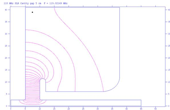
Figure 3: The SPS-II 119 MHz cavity profile.
