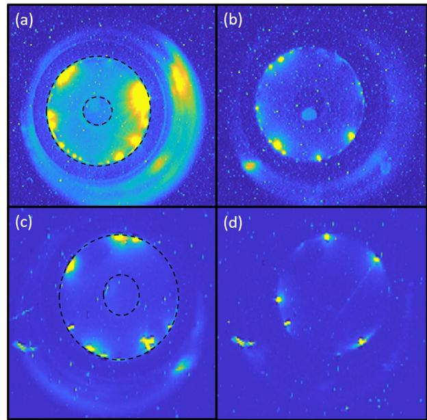
Figure 3: Snapshots of the face of the upstream (a & b) and downstream (c & d) disks, taken at the beginning (a & c) and end (b & d) of conditioning. The extents of the ceramic marked with dashed black lines on the left.
