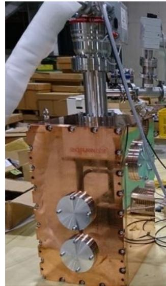
Figure 6: Assembled cavity after second machining.
