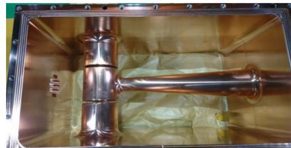
Figure 4: Buncher main body after first machining and Assembled cavity inner dimension.
