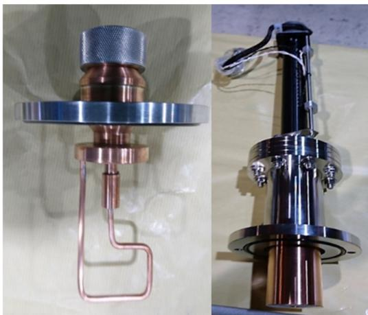
Figure 5: Power coupler (left) and tuner (right).
