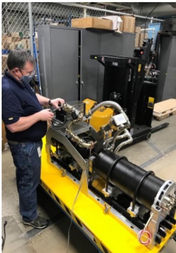
Figure 3: New 10 MeV S-Band ABC for high e-beam power applications.
