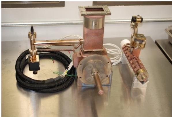
Figure 1: 3 MeV S-Band and 3 MeV X-Band ABC (at the correlated RF power settings). Note difference in radial dimensions for the two ABCs.
