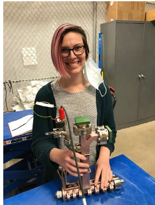
Figure 3: Two section X-band ABC, designed to operate at 2.5 MeV and dose rate up to 50 R/min @1 m from target.
