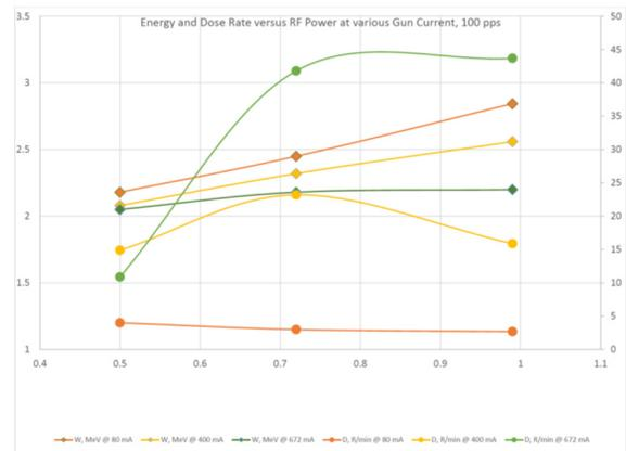
Figure 5: ABC-1.8-X-X test results with higher power magnetron, at 100 PPS in a range of injected current.
