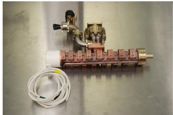
Figure 2: Single section X-band ABC, designed to operate at 1.8 MeV and at 2.5 MeV at 350 kW and 700 kW RF power input, correspondingly.
