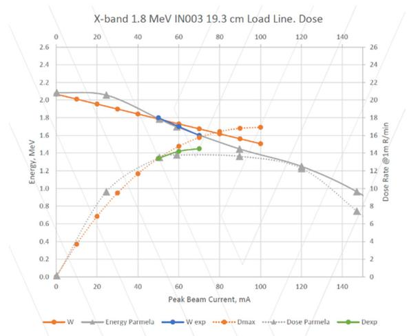
Figure 4: ABC-1.8-X-X design and experimental results using 350 kW peak RF power magnetron.
