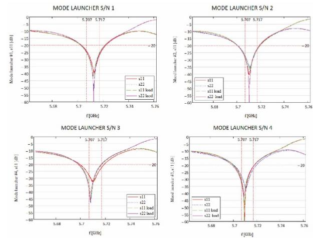
Figure 4: Reflection characteristics measured for the four fabricated mode launchers.
