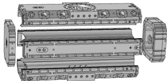
Figure 2: Exploded view of segment 1 with the plunger cover used for RF tests.
