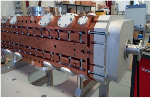
Figure 3: Segment 1 with the plunger cover in position, ready for RF tests.
