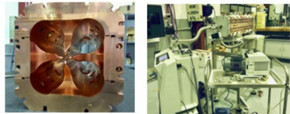
Figure 1: Left: A picture of the assembly of segment 1 of the RFQ. The channels for the O-rings and for the RF contacts can be seen. Right: Vacuum leak tests of segment 1.
