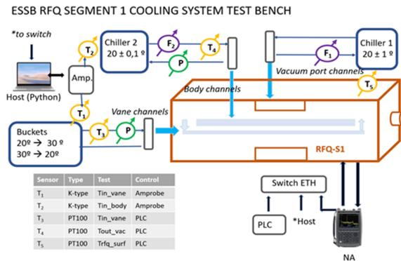
Figure 6: Schematic of the experimental setup for the frequency measurements as a function of cooling water temperature.
