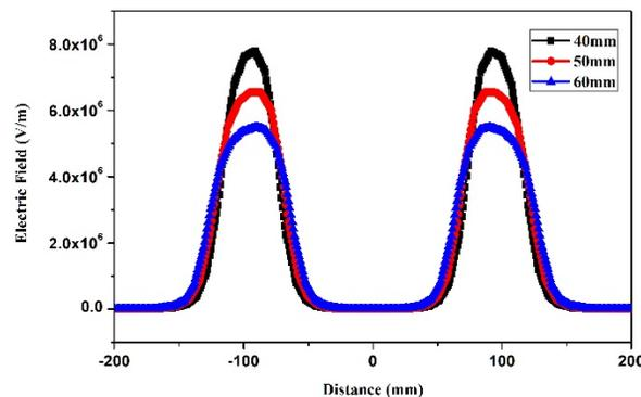
Figure 6: The electric field pattern along the beam direction when the gap has been varied from 40 mm to 60 mm.
