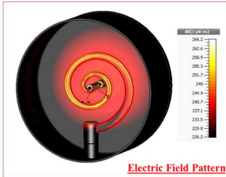
Figure 2: The electric field intensity along the spiral type central conductor.
