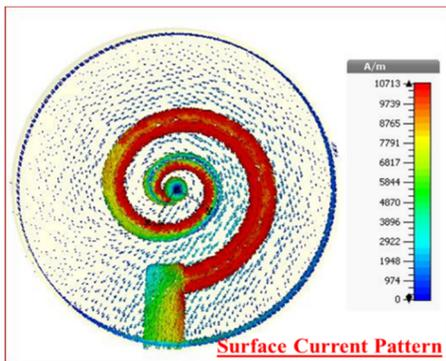
Figure 4: The surface current intensity along the spiral type central conductor.
