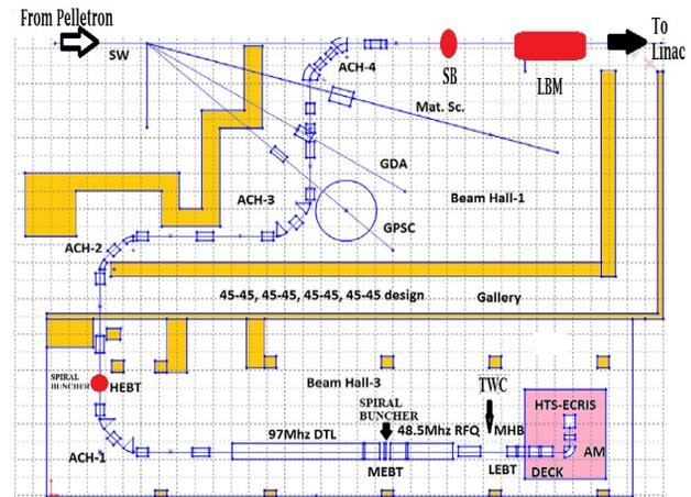
Figure 1: The pictorial layout of the high current injector accelerator.
