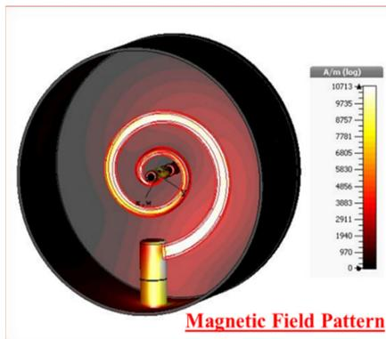
Figure 3: The magnetic field intensity along the spiral type central conductor.
