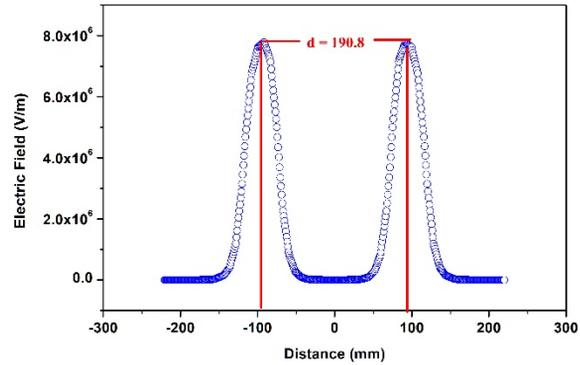
Figure 5: The electric field pattern along the beam direction of the buncher cavity.
