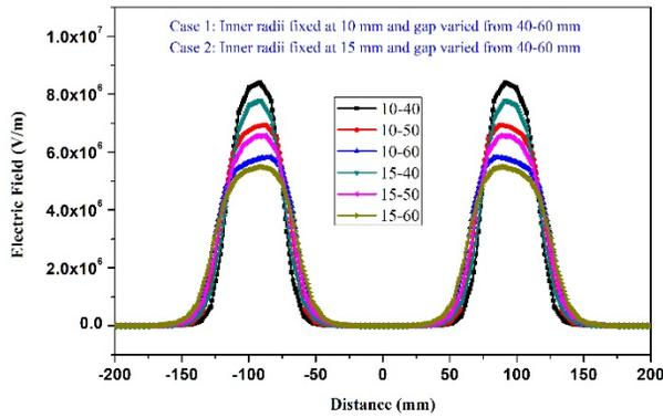
Figure 7: The electric field pattern along the beam direction when the inner and outer radii have been varied.
