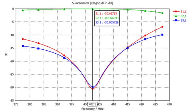
Figure 2: Frequency Domain Response of the DTL Circulator after Tuning.
