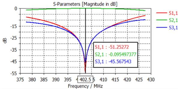
Figure 4: Frequency Domain Response of the DTL Circulator after Tuning (Optimal Tuning Case) [3].
