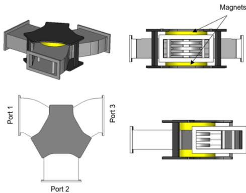
Figure 1: 3-D Model of the SNS DTL Circulator. [3]
