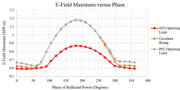
Figure 5: Maximum E-Field Intensity as a Function of the Transmitted Power Phase (Optimal Tuning Case) [3].
