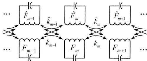
Figure 2: Equivalent circuit representation:  $m$  is the cell index,  $F_m$  is the single cell frequency,  $k_m$  the coupling constant between two adjacent cells. The quantities with the symbol “^” refer to the TE mode.
