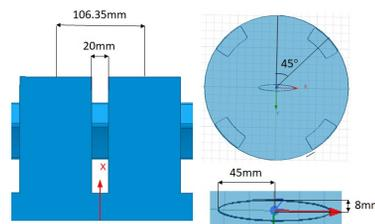
Figure 1: Standard cell with its main parameters.
