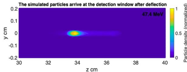
Figure 7: The simulated longitudinal profile of the beam.
