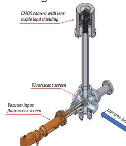
Figure 2: Scheme of fluorescent sensor in SKIF linac.
