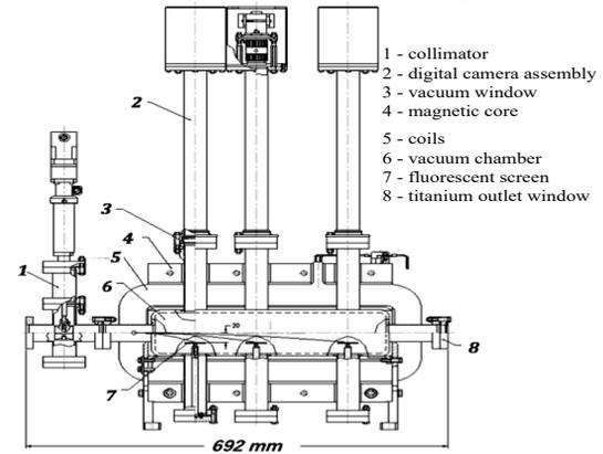
Figure 6: Layout of magnet spectrometer.
