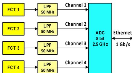
Figure 8: Block diagram of beam charge measurements.
