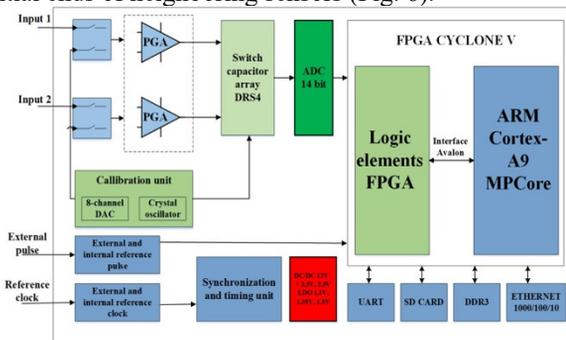
Figure 5: Simplified diagram of the measurement module for CBLM.
