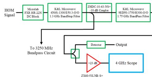
Figure 1: Block diagram of the 1750 MHz section of the Fermilab Prototype. This includes an amplifier (red) added for the February 2020 experiment.
