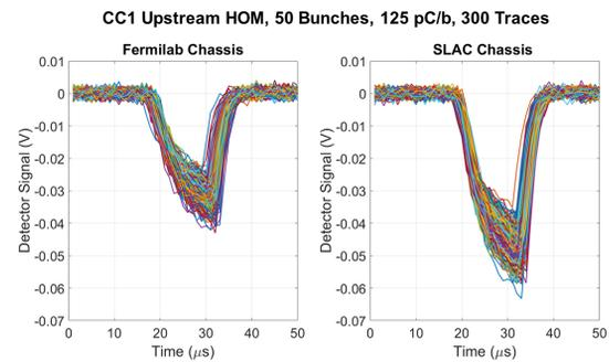
Figure 4: Overlay of 300 traces of CC1 data taken under the same beam conditions with the Fermilab and SLAC prototypes. The electron beam is 50 bunches at about 125 pC/bunch with a spacing of 333 ns.
