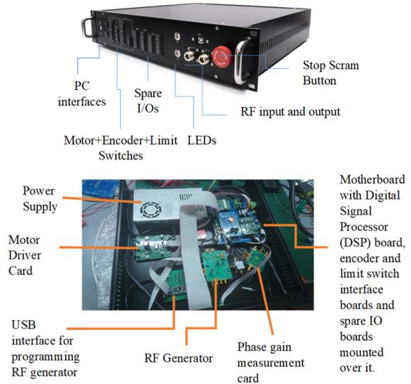
Figure 4: Major components of the bead-pull control system.
