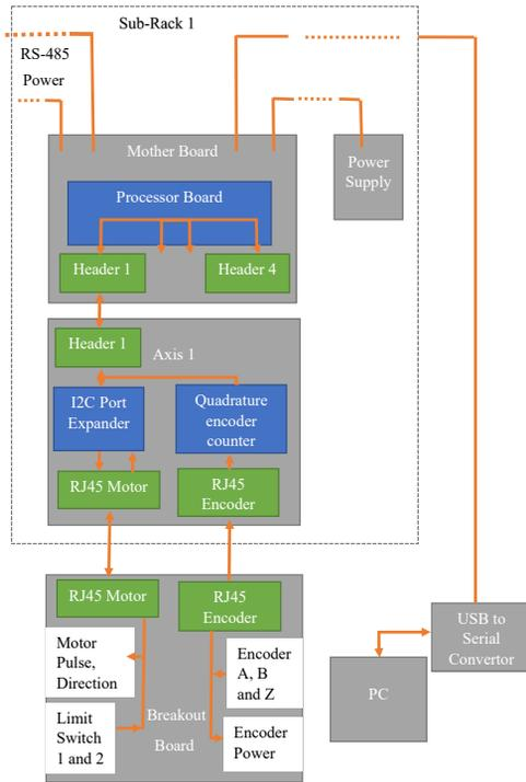
Figure 2: Architecture of the 64-axis motion controller.
