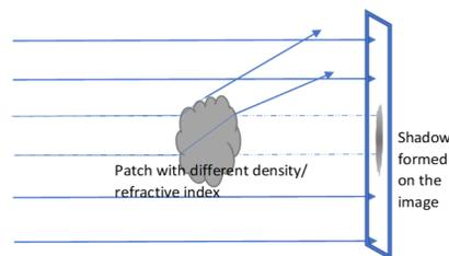
Figure 1: Formation of shadow image of gas flow.
