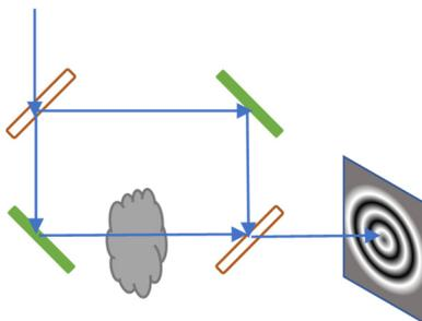
Figure 3: Formation of interference image of gas flow.
