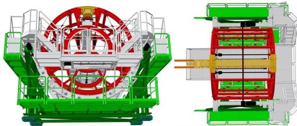
Figure 6: Rear and top views of the new Enfourneur 3D CAD model with electrical motors, translation screws and rack integrated (darkest parts).
