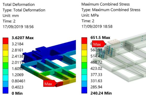
Figure 3: Maximum combined stress calculated on the screws with preload applied on the new rear low balcony.
