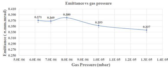
Figure 7: Result plot emittance vs operating gas pressure.
