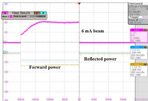
Figure 5: Beam pulse on faraday cup.
