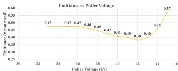
Figure 6: Plot of emittance vs puller electrode potential.
