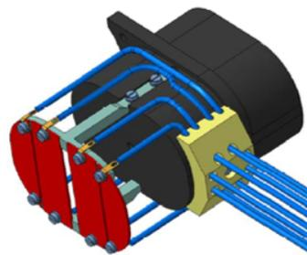
Figure 4: PSB  $\text{H}^0$ - $\text{H}^-$  beam current monitor installed after the  $\text{H}^-$  stripping foil units: four plates integrate the signal from non stripped ions before they are absorbed by the dump.
