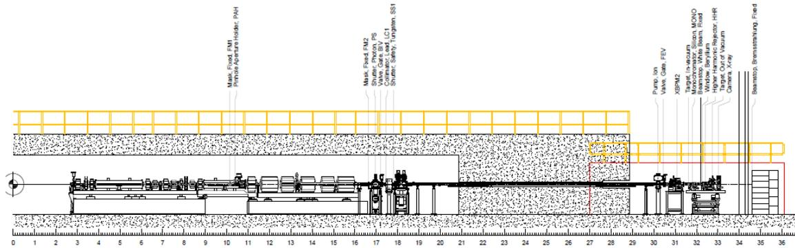
Figure 1: Elevation view of APS-U beam size monitor beamline. Principal beamline components are annotated. The longitudinal coordinate is metres from the centre of the insertion device straight. The bending magnet photon source point is at 3.83 m. The extent of the new BSM beamline enclosure is outlined in red.
