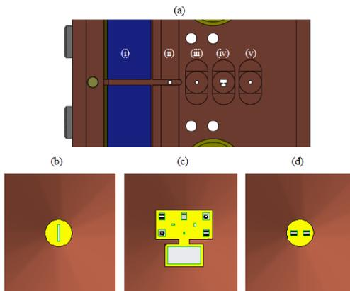
Figure 2: PAH and apertures. (a) Overview of apertures in PAH. (i) XBPM1 electrodes (in blue). (ii) BL1 (beam-defining aperture for XBPM2). (iii) BL2. (iv) BL3. (v) BL4. (b) Enlarged image of BL2 slit defining horizontal relative beam size monitor. (c) Enlarged image of BL3 apertures defining absolute beam size monitor. (d) Enlarged image of BL4 apertures defining vertical relative beam size monitor.
