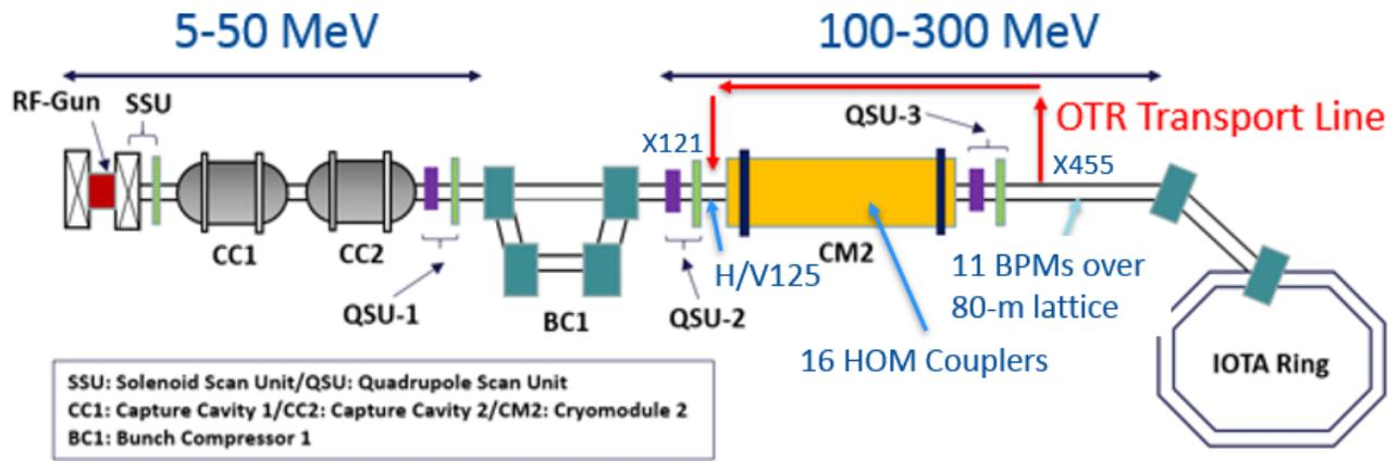
Figure 1: Schematic of the FAST/IOTA beamline layout.
