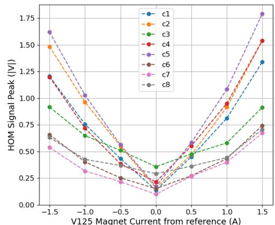
Figure 3: HOM peak signals vs V125 corrector current values for different values of V125 with 400 pC/b, 50 b and H125 at reference value.
