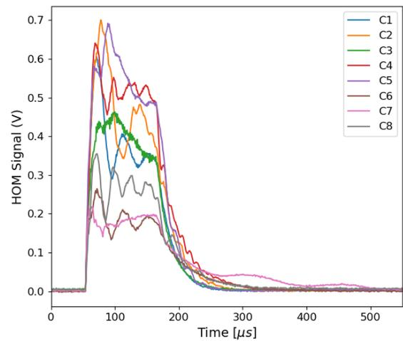
Figure 2: US HOM waveforms with 125 pC/b, 50 bunches, V125=+1.0 A and H125 at reference value.
