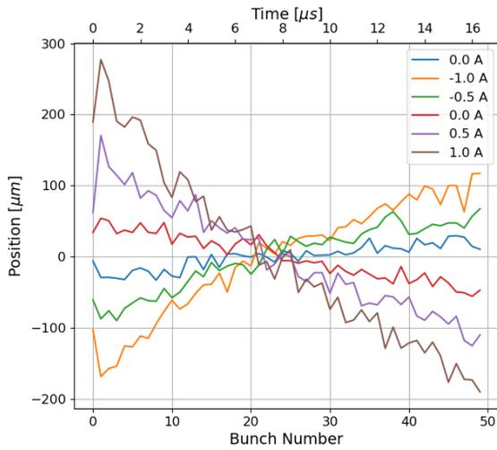
Figure 4: Bunch by bunch centroid slew in B441PV for different values of V125 corrector current offset, with 125 pC/b, 50 bunches and H125 at reference value.
