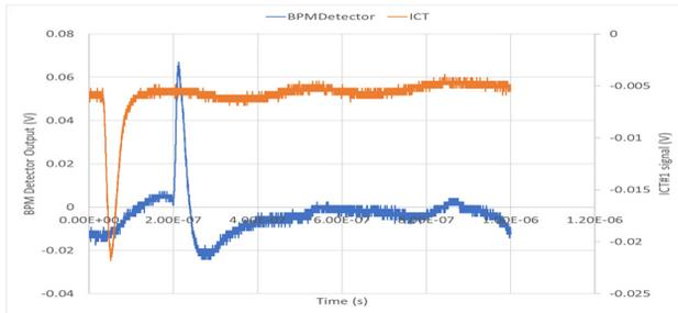
Figure 8: 2SC4083 active-filter output response to button BPM with 500 pC charge.
