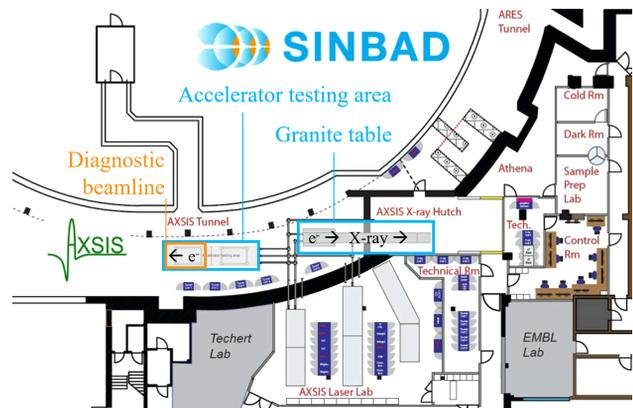
Figure 1: Floor plan of the AXSIS facility. The accelerator testing area with the electron diagnostic beamline and the granite table for the final accelerator installation are highlighted. “Figure 2” by [4, p. 3598], used under CC BY 3.0 [5]. Highlighting and annotations added to original.
