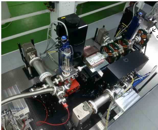
Figure 3: Photograph of the installed electron diagnostic beamline in the AXISIS tunnel. The beam enters from the right.
