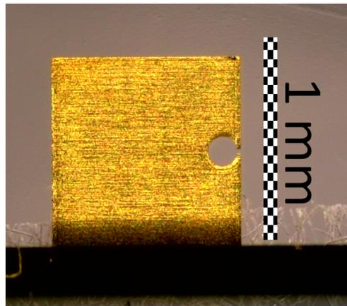
Figure 1: Image of the split-ring resonator device. The streaking EM field is located in the split of the ring with a size of  $20\ \mu\text{m}$  by  $20\ \mu\text{m}$ .
