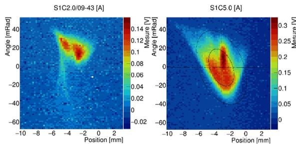
Figure 3: (x,x') Distribution of the H<sup>-</sup> beam. On the left, the source current (S1C) is fixed at 2 A. It is the start-up reference beam. On the right, one of the measurements for the arc current ramped up to S1C=5 A. Also, 1 and 2- $\sigma$  ellipses are drawn, with the centroid (cross).
