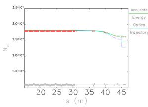
Figure 4: Beam losses in the electron injection channel.
