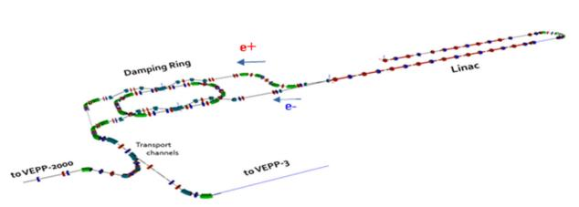
Figure 1: The layout of Injection Complex VEPP-5, its components and initial sections of the transport channels to colliders VEPP-4M and VEPP-2000.
