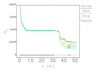
Figure 3: Beam losses in the positron injection channel. Thick green line is for the best optimized beam transportation with no errors.
