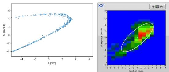
Figure 4: Comparison of the simulated (left) and measured (right) beam emittance at the end of the HRS. This has been simulated with COSY and confirmed by Zgoubi. This figure has been obtained by turning off the last doublet of quads in the beamline so that the beam is large enough to be measured. The tail on the left of the simulated emittance also disappears when a binning and a threshold are applied on the simulated data as for the experimental data.
