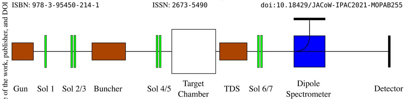
Figure 1: Schematic overview of the REGAE beamline featuring the rf cavities (brown), magnetic solenoids (green), dipole spectrometer (blue) and detector screens (black). The position of the target chamber is also indicated.
