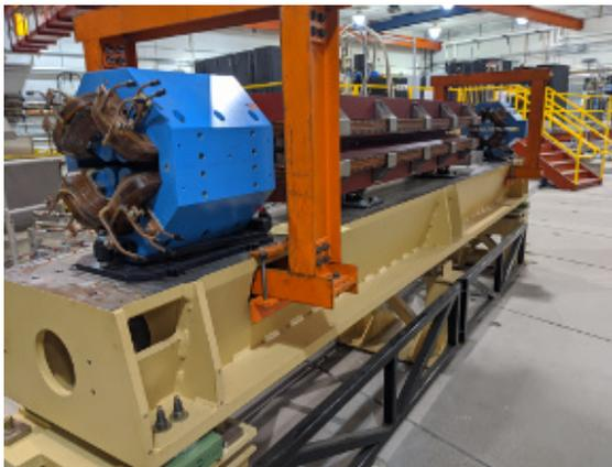
Figure 1: Photograph of one half of the double achromat cell used in the 2018 upgrade of the south arc of the CESR ring.
