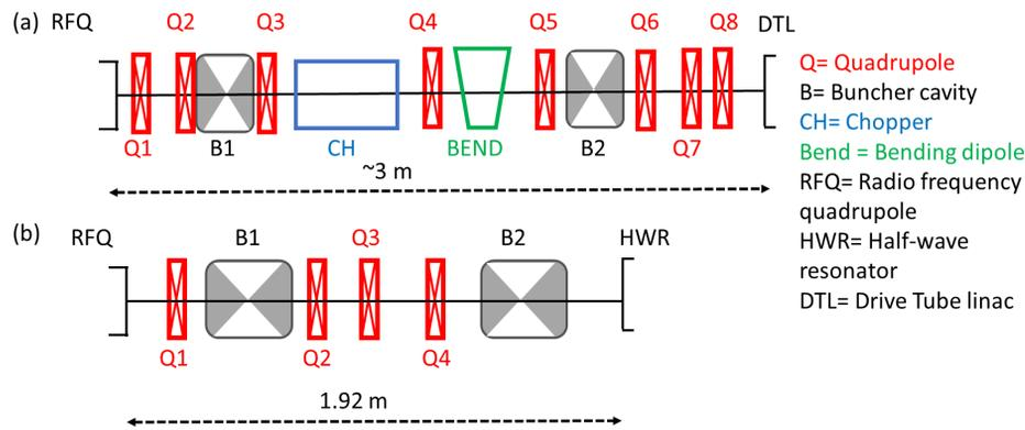
Figure 2: MEBT lattice design for the J-PARC linac (a) and the JAEA-ADS (b).
