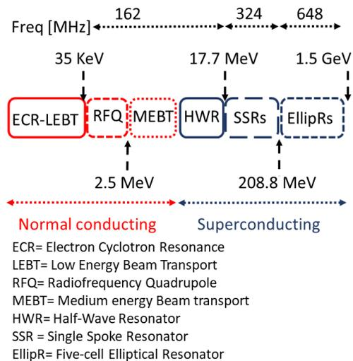
Figure 1: Schematic design of the JAEA-ADS linac.
