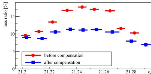
Figure 3: Measured beam loss ratio before (red) and after (blue) the compensation in each tune [4].
