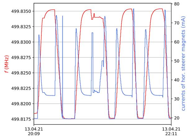
Figure 4: Measured rf frequency  $f$  and total horizontal steerer currents while switching between optic settings with method II.
