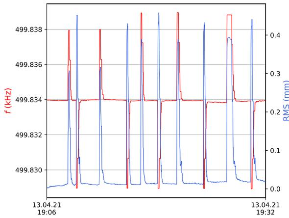
Figure 2: Measured rf frequency  $f$  and RMS orbit deviation while applying method I.
