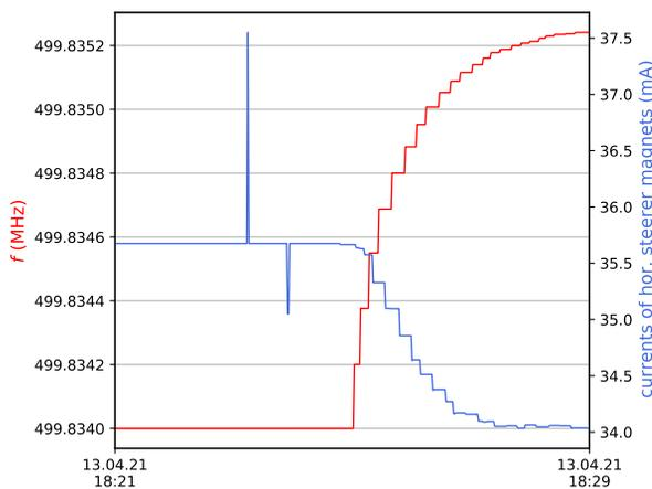
Figure 3: Measured rf frequency  $f$  and total horizontal steerer currents while applying method II at user orbit. The two spikes are measurement artifacts.
