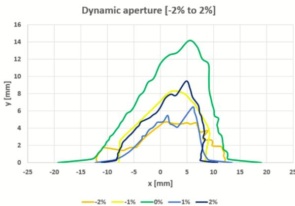
Figure 5. An optimized dynamic aperture of 4GSR.
