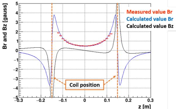
Figure 3: Calculation results of the magnetic field distribution created by the kicker coil and the radial magnetic field distribution measured by the pickup coil.
