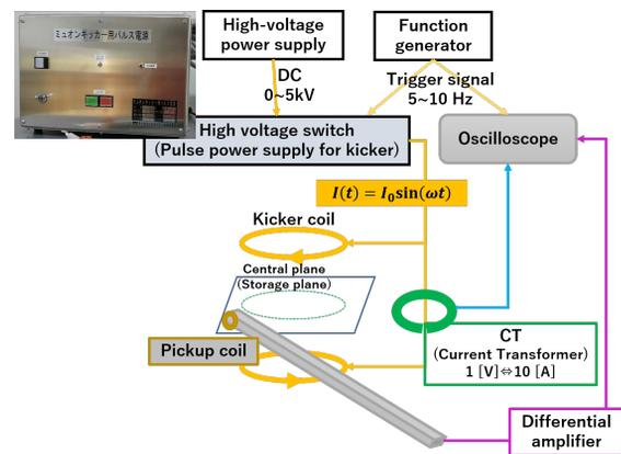
Figure 4: Experimental setup for stand-alone performance evaluation measurement.
