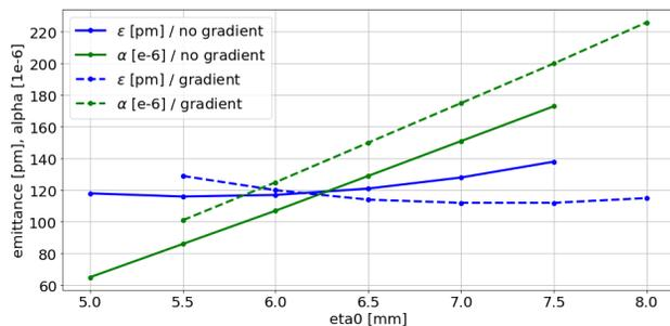
Figure 3:  $\epsilon$  and  $\alpha$  as a function of  $\eta_0$  for a homogeneous dipole (line) and a gradient dipole (dashed) with  $L/2 = 0.6$  m. The  $\epsilon$  gain due to the gradient becomes relevant for large  $\eta^0$ .
