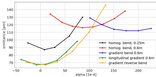
Figure 4:  $\epsilon - \alpha$  pairs achievable with 5 UCs, utilizing different magnets. Different hardware solutions support either large  $\alpha$  or small  $\epsilon$ . Combinations are possible.
