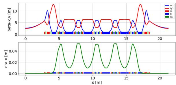
Figure 6: An example lattice for BESSY III, with gradient-free, long dipoles in the UC, but gradient bends in the MC.
