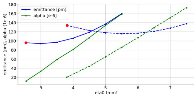
Figure 2: Longer dipoles:  $\epsilon$  and  $\alpha$  as a function of  $\eta_0$  for a half dipole length of  $0.4$  m (line) and  $0.6$  m (dashed). Red dots indicate the values for  $\eta^{0,TME}$ , clearly off  $\epsilon_{min}$ .
