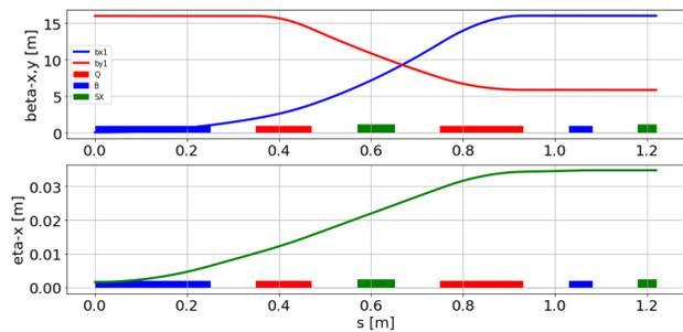
Figure 1:  $\beta_{x,y}$  (top; blue, red) and  $\eta$  (bottom, green) of the most basic (half) unit cell seeking minimal emittance and length and obeying given field constraints. Dipoles are blue, quadrupoles red and sextupoles green.
