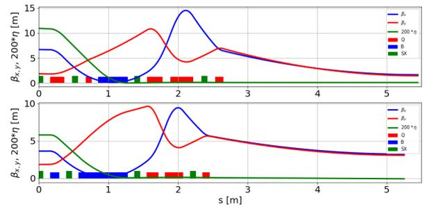
Figure 5: Dispersion matching with 2 quads and the bend gradient (top); and with the length and gradient of the dipole, (bottom). Full linear control depends on 6 free parameters.
