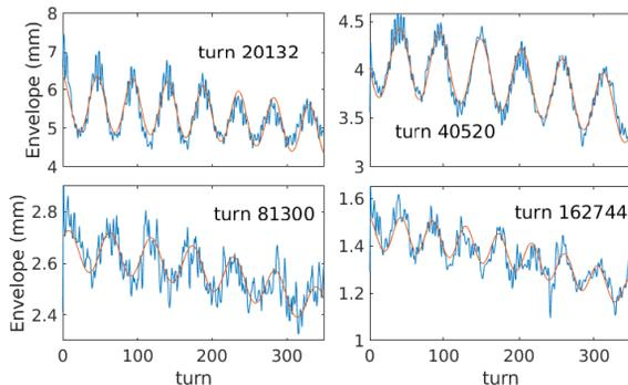
Figure 8: Fitting horizontal oscillation envelope to Eq. (2) for four points on the ramp.
