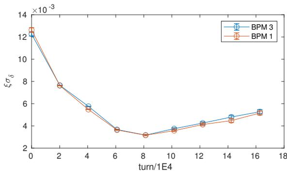
Figure 9: Fitted  $\xi\sigma_\delta$  on the ramp with data from two BPMs.
