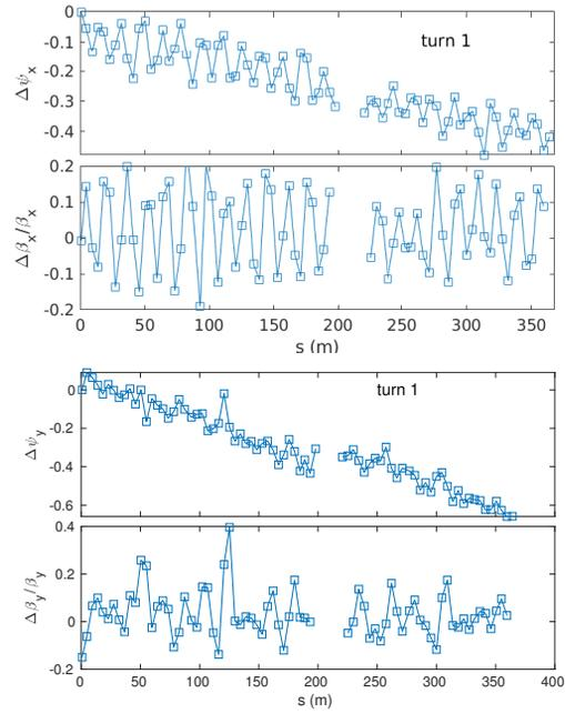
Figure 4: Horizontal (top) and vertical (bottom) phase advance obtained with ICA and the corresponding beta beating derived with the 3-BPM method, at injection.
