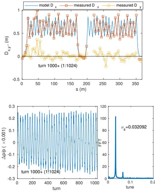
Figure 3: The dispersion functions (top) and the corresponding momentum deviation oscillation (bottom) measured 1000 turns after injection.
