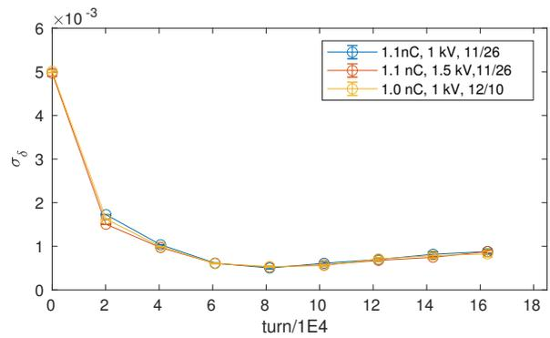
Figure 10: The beam momentum spread on the energy ramp for the APS Booster measured from decoherence for three data sets, with bunch charge and kicker strength indicated in the legend.
