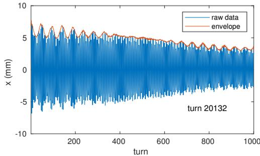
Figure 7: Horizontal BPM data after the kick at turn 20132 observed at one BPM, with oscillation envelope.
