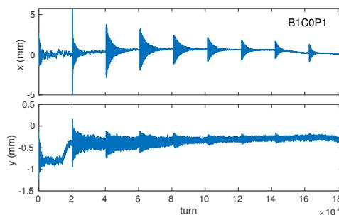
Figure 2: Horizontal (top) and vertical(bottom) BPM data on the ramp of the APS Booster observed at one BPM. Horizontal motion was excited by the extraction kicker.
