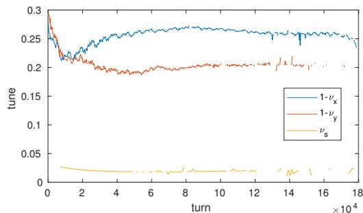
Figure 1: Betatron and synchrotron tunes on the Booster energy ramp measured by TBT BPM.
