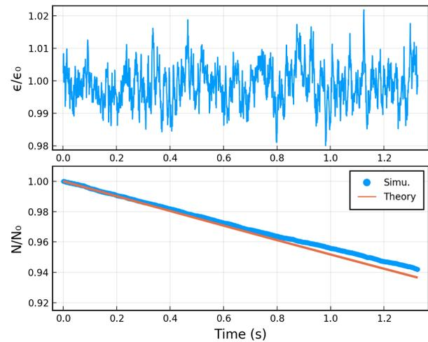
Figure 1: Evolution of beam emittance and particle number in the 1-d tracking ( $A = 4.6$ ,  $\lambda = 100 \text{ s}^{-1}$ ,  $\tau_{theory} = 18.6 \text{ s}$ ).
