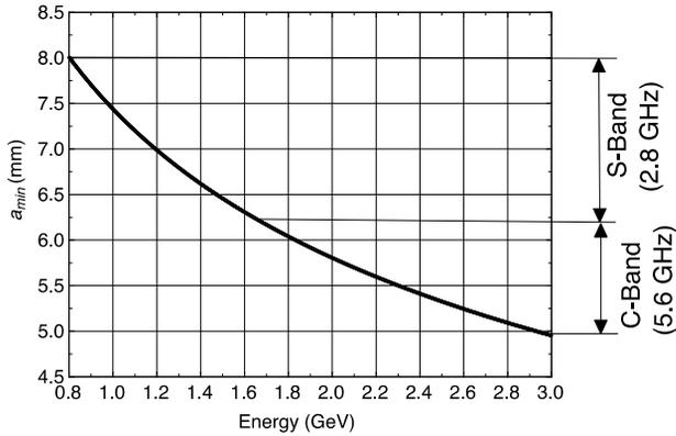
Figure 1: Minimal cavity aperture vs beam energy.
