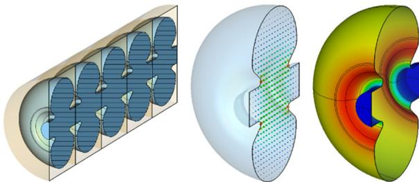
Figure 5: S-band structure for  $\beta=0.84$  (left to right): 5-cell structure section; electric field within a cell; current distribution on the cell inner surface.
