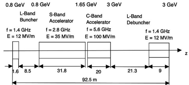
Figure 3: Layout of 3-GeV HG pRad booster.
