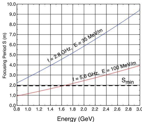
Figure 2: Maximal focusing period vs beam energy.
