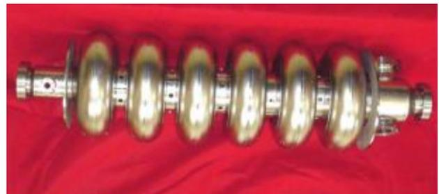
Figure 1: SNS linac superconducting cavity.
