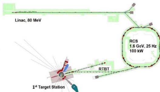
Figure 1: Schematic diagram of CSNS.
