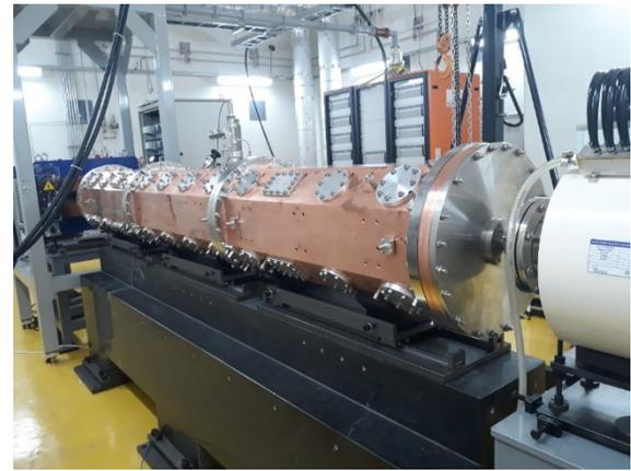
Figure 4: Installed RFQ.
