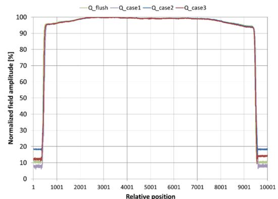
Figure 5: Quadrupole field profile (flush: all tuners are design position, case1: first iteration, case2: second iteration, case3: third iteration).
