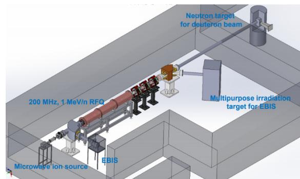
Figure 1: Layout of the 1 MeV/n RFQ system.
