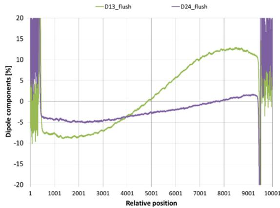
Figure 6: Dipole field profile (flush: all tuners are design position).
