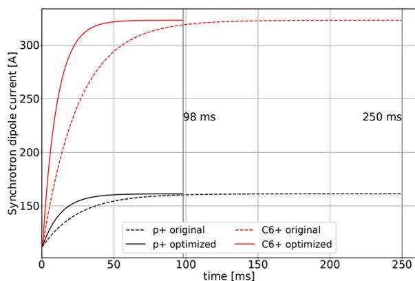
Figure 2: Current ramp of the synchrotron dipoles for protons and carbon ions before and after the injection timing optimization.
