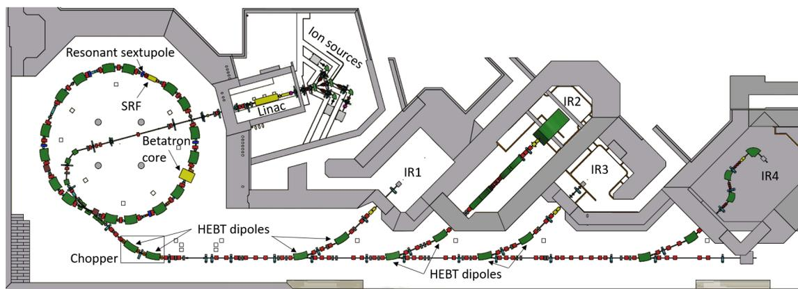
Figure 1: Layout of the MedAustron accelerator complex.
