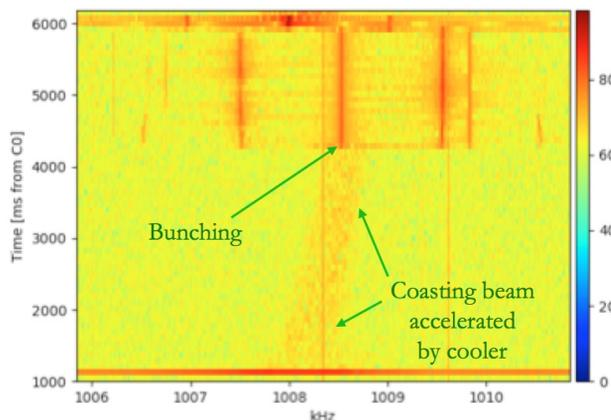
Figure 6: Longitudinal Schottky spectra of a coasting  $H^-$  beam under electron cooling.
