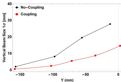
Figure 5: The comparison of vertical beam size with and without XY-coupling. The vertical beam size at the kick point ( $Y \approx -100$  mm) was  $8.18 \pm 0.03$  mm ( $1\sigma$ ) without XY-coupling, which has been controlled to  $2.56 \pm 0.005$  mm ( $1\sigma$ ) with appropriate phase space matching.
