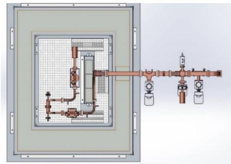
Figure 6: The top view of the waveguide assembly for the CERF-NM Test Stand. The assembly of two Mode Launchers (Mode Converters) at the end of the waveguide is shown on this figure. Courtesy of Harbhajan Khalsa.
