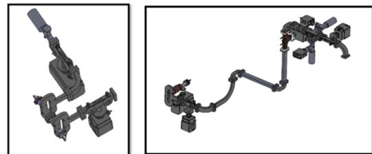
Figure 7: Left – two Mode Launchers back-to-back setup for conditioning and conversion efficiency check. Right – test run setup with single Mode Launcher and RF cavity.
