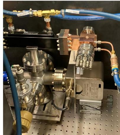
Figure 11: First cavity is being tested in the Test Stand. This is OFHC Cu cavity from our collaborators at SLAC, designed for acceleration of protons/ions at relative velocity of 0.5 of the speed of light.
