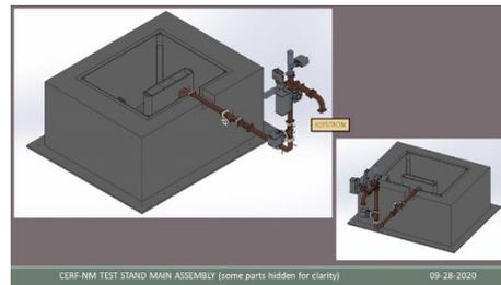
Figure 5: The 3D view of the waveguide assembly for the CERF-NM Test Stand. Courtesy of Harbhajan Khalsa.
