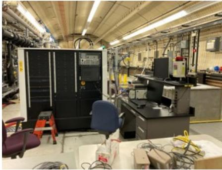
Figure 2: View of the tunnel. Foreground – computer control station. Left – C-band klystron. Right, background – lead enclosure.
