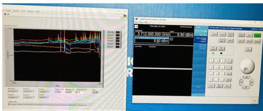
Figure 10: Typical computer control screen during waveguide conditioning. On the left is the window with the pressure measurements curves in different points along the waveguide line. On the right is the RF power control window.
