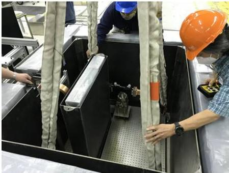
Figure 9: Second segment of the waveguide is installed inside the lead enclosure and later is connected to the first segment.
