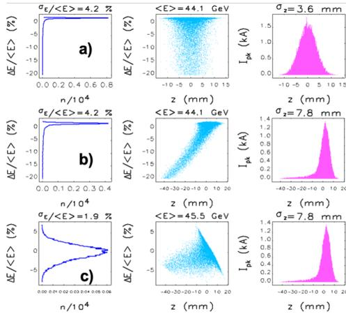
Figure 3: Longitudinal phase space distribution of the  $e^+$  beam in the compressor linac: a) at the entrance of the matching section upstream the magnetic chicane, b) at the exit of the chicane, c) at the exit of the linac.
