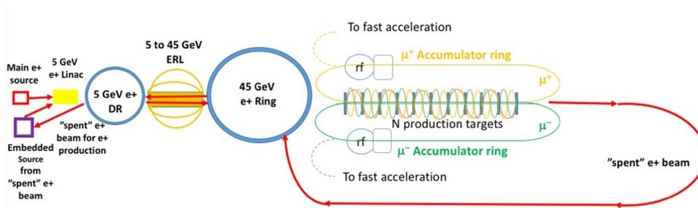
Figure 1: The LEMMA positron driven muon source.
