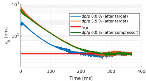
Figure 4: Horizontal injected beam emittance after injection in the PR with the initial beam distribution after the targets (blue, orange) for two different injected beam energy offsets, and after the linac compressor (green).
