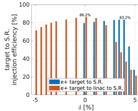
Figure 5: Injection efficiency vs beam energy offset, for the beam distribution after the targets (blue) and after compressor linac (red).
