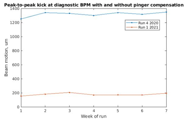
Figure 7: Peak-to-peak stored beam motion monitored over 7 weeks. Blue shows a run without PMs operating, red shows a run with PMs operating.
