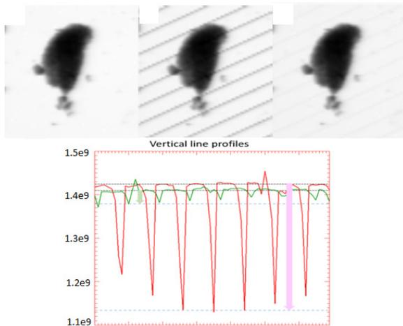
Figure 2: Top: Raster scans in I08 with no disturbance (left), injection magnets (middle), and both PMs (right). Bottom: Vertical slices through the middle (red) and right (green) plots.
