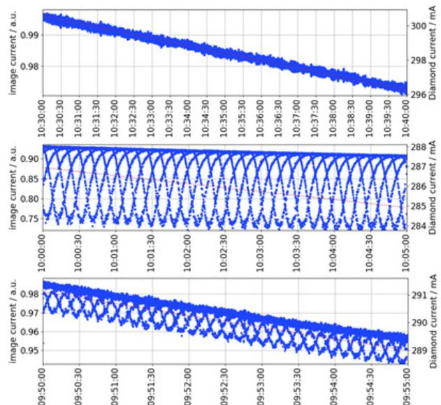
Figure 4: Image current at mirror with no disturbance (top), injection magnets only (middle) and injection magnets with both PMs (bottom).
