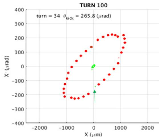
Figure 1: Measured bunch phase space (red) and simulated phase space after correction (green).
