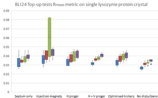
Figure 6: Rmeas statistic plotted for the various test schemes as indicated in Table 1.
