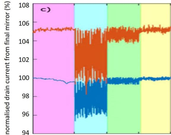
Figure 3: Intensity for hard (red, offset by +5%) and soft (blue) x-rays with no disturbance (left, pink), injection magnets only (centre-left, cyan), injection and horizontal PM (centre-right, green) and injection and both PMs (right, yellow).
