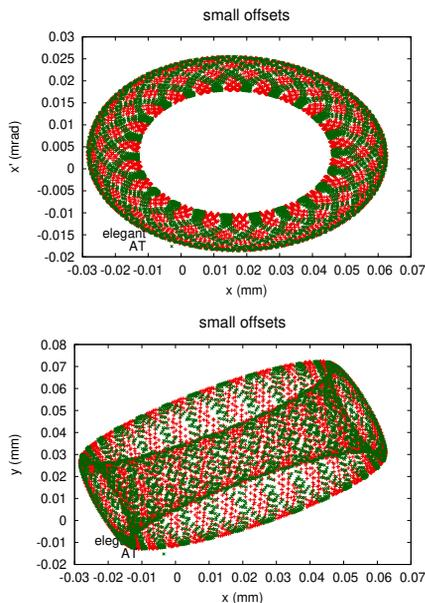
Figure 4: Comparison of turn-by-turn particle trace in AT and elegant, for small offset errors, in phase space (top) and coordinate space (bottom).
