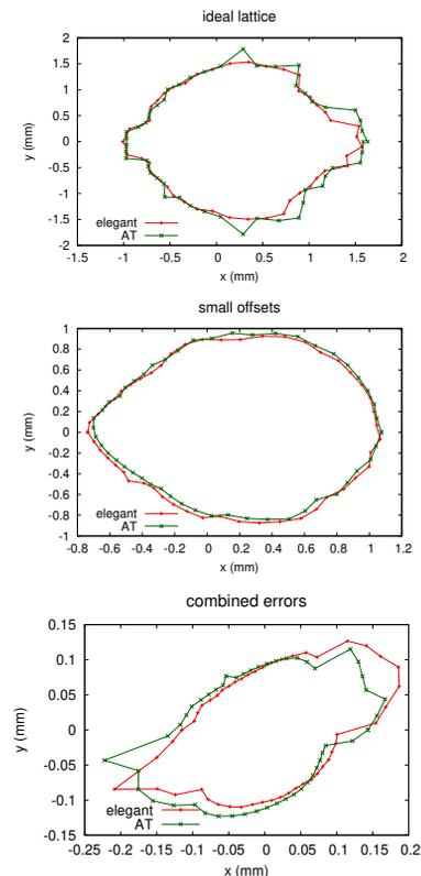
Figure 5: Dynamic aperture in AT and elegant, for three lattices with varying error models.
