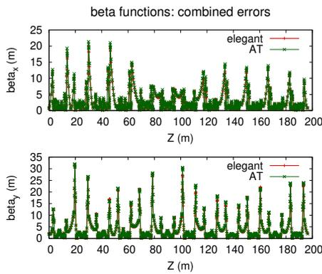
Figure 2: Comparison of beta functions in AT and elegant, for several error types combined.
