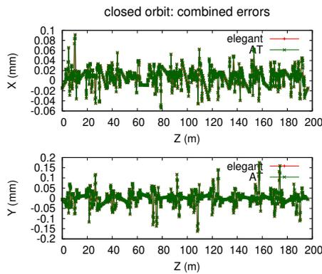
Figure 3: Comparison of closed orbit in AT and elegant, for several error types combined.
