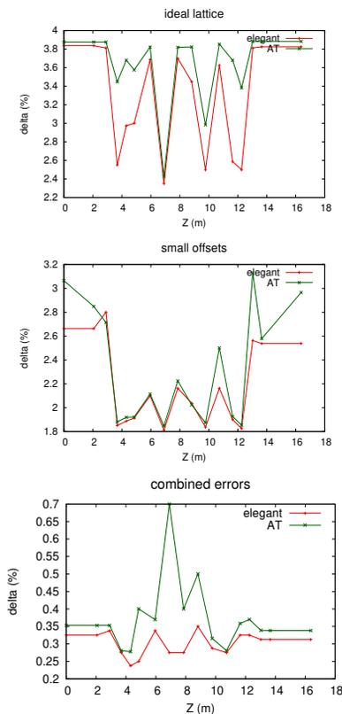
Figure 6: Momentum aperture in AT and elegant, for three lattices with varying error models.
