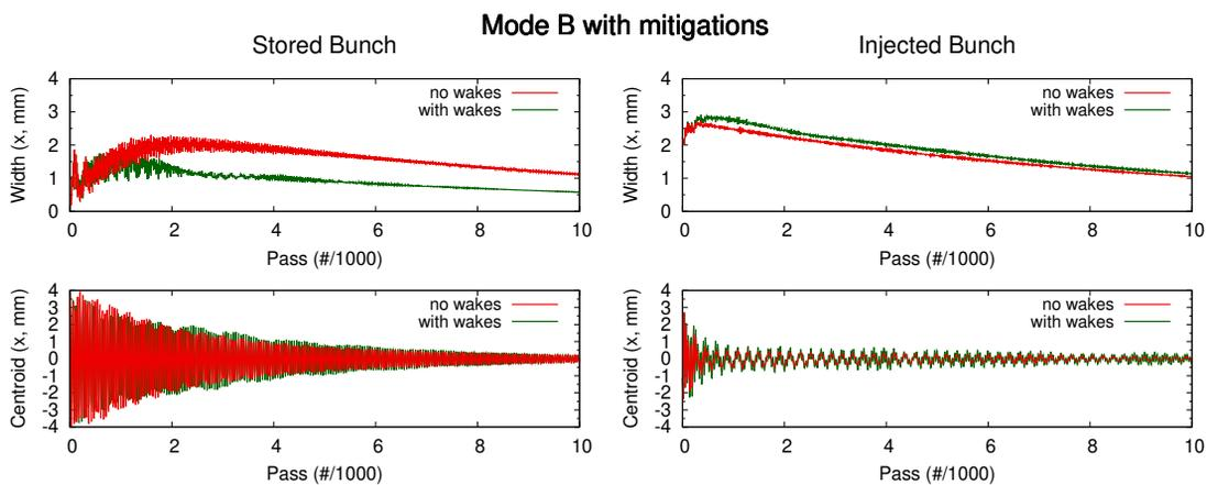
Figure 4: Dynamics of the stored and injected bunches without wakes (red) and for the nominal wakes (green), in the Mode B configuration with chromaticity increased to 1.2 and a time delay of 100 ps.
