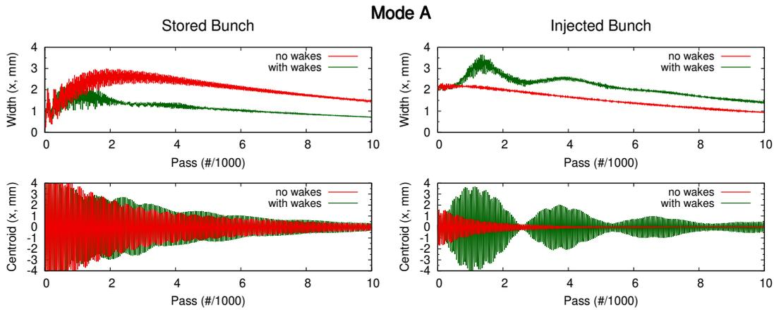
Figure 3: Dynamics of the stored and injected bunches without wakes (red) and for the nominal wakes (green), in the Mode A configuration.
