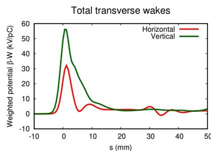
Figure 1: Transverse short-range wake field potentials for the ALS-U accumulator ring.
