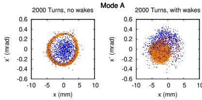
Figure 2: Distribution of the stored (orange) and injected (blue) electrons in the Mode A configuration after 2000 passes around the ring, both without (left) and with wakes (right).
