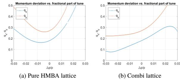
Figure 4: Fractional part of the tune as a function of the relative momentum deviation.
