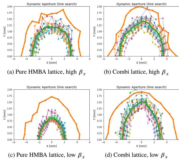
Figure 5: Dynamic aperture at the injection point ( $\beta_x = 21.7$  m,  $\beta_y = 3.7$  m) with errors and without (orange line).
