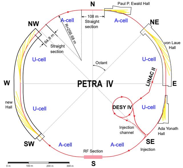
Figure 1: Layout of PETRA IV. The positions of the undulator cells (U-cell) and the relaxed cells (A-cell) for the combi lattice are marked in blue. The pure HMBA lattice is using U-cells for all arcs.
