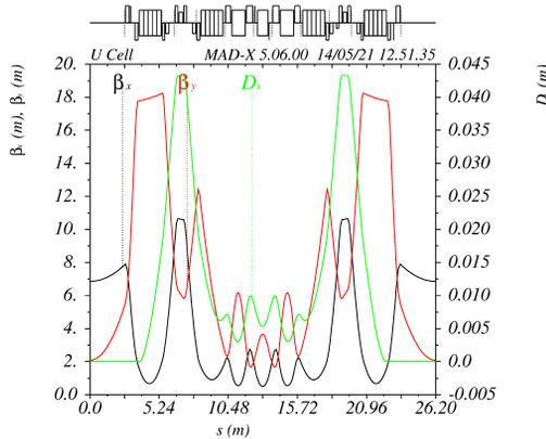
Figure 2: HMBA cell for arcs with undulators (U-cell).
